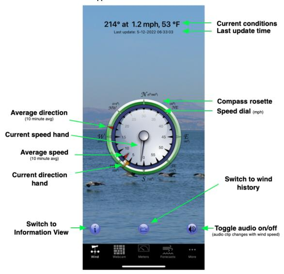
The view consists of two concentric dials and four dial hands. The outer dial is the compass rosette, while the inner dial is the speed dial.
