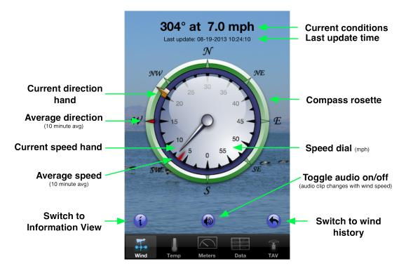
The view consists of two concentric dials and four dial hands. The outer dial is the compass rosette, while the inner dial is the speed dial.
