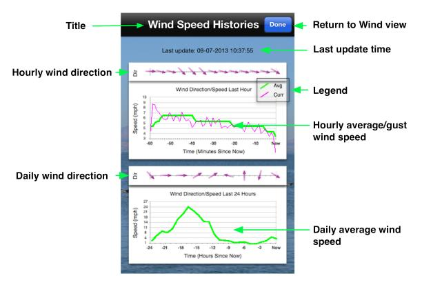
There are two graphs for each view, one representing direction and one representing speed. On the hourly view there will be two plots, one representing the average wind speed (in green) and one representing the instantaneous or 2-minute gust speed (in purple).
